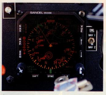
With two Garmin 430s, an UPSAT MX20 multifunction display, and a Sandel EHSI (electronic horizontal situation indicator), this Aztec is uniquely display-heavy.
