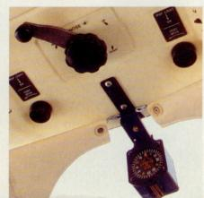
Aztec baggage capacity is 300 pounds, split between the nose and aft baggage compartments. The overhead pitch- and rudder-trim cranks can give neophytes fits. Electric pitch trim can do away with the "wrong way" manual cranking problem. Approaches can be flown at 90 KIAS or 100 mph using full flaps. With minimal experience, you can easily learn to consistently make greaser Aztec arrivals.
